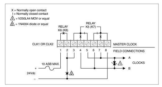
Figure B-15 Two-Wire Pulse Alternating (24Vdc)
